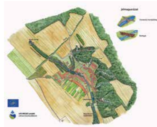
25 – Visual design of envisaged run-off deceleration solutions in the upper catchment area of Creek Szilágyi. (Designer: Csilla Ruzics)
