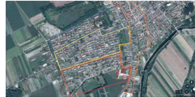
18 – Areas from which rainwater is collected in the reservoir in Bática, by implementation phase. (Source: Google Earth)
