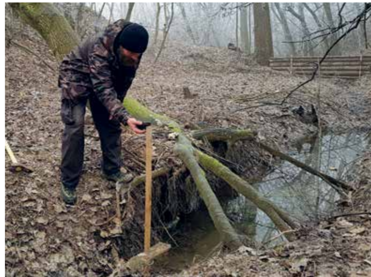
54 – A simple measuring system to monitor how the storage basins above the log dams installed in the erosion gully are silting up. (Photo: WWF HU.)
